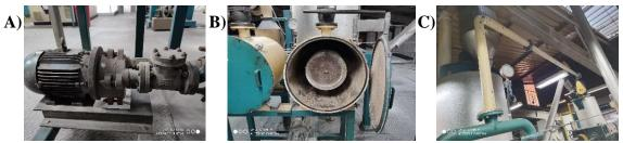
Fig. 1: PET extruder vacuum system. a) Air pump, b) Vacuum system, c) Pipe system.
