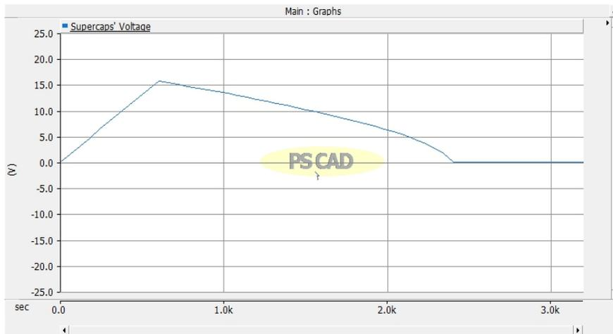
Fig. 3 20F bank charge and discharge curve
