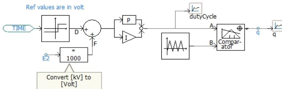
Fig. 2 Controller of buck-boost converter
